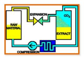
an condenser, compressed in an circulating pump, heated and fed back to the extractor. This completes the process that operates in a closed circuit consisting of intake-compression-extractionexpansion-condensation-intake. All process side parts are made of stainless steel.
